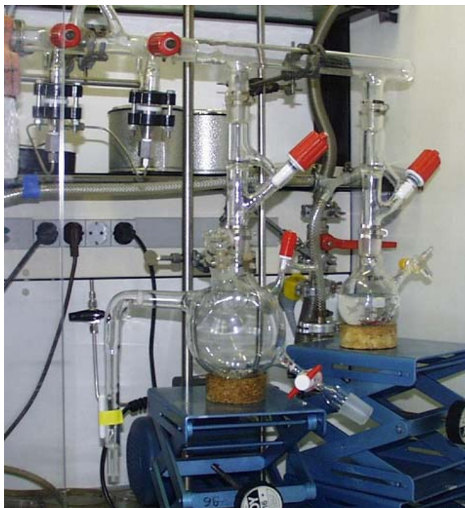
Figure 3. 3. Glass reactor used for the UV-visible spectroscopy study.
