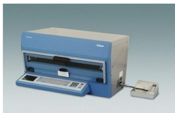
Figure 11. Schematic representation of a panel test (lines delimit temperature segments but are only drawn to facilitate visualization) and gradient –oven (BYK Gardner)
