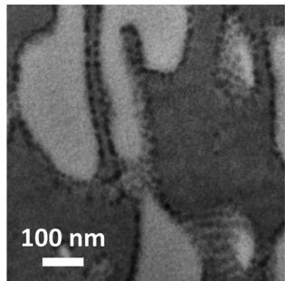
**Figure 3.** TEM micrograph illustrating the densely packed structure of the SBM JPs at the PS:PMMA interface in a 44:56 PS:PMMA + 20 vol % SBM JP blend. The center-to-center distance is about 20 nm, while the particle cores are separated by 10 nm, approximately twice the size of the grafted chains.
