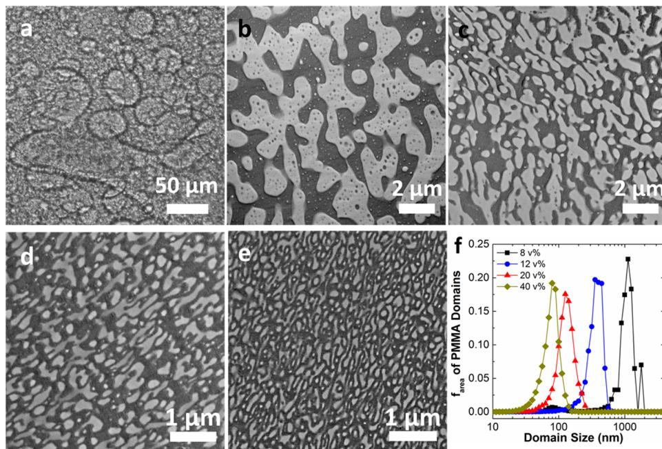
**Figure 2.** (a–e) Images demonstrating the change in domain size with varying loadings of SBM JPs in 44:56 PS:PMMA (as cast). (a) Optical image of blend with 0 vol % SBM JP, and TEM micrographs of blends with (b) 8, (c) 12, (d) 20, and (e) 40 vol % SBM JP loadings. The dark gray phase in the micrographs is PS; the light gray phase is PMMA. (f) Histogram plot of the area-weighted fraction of PMMA domains as a function of domain size (chord length), as determined by image analysis.
