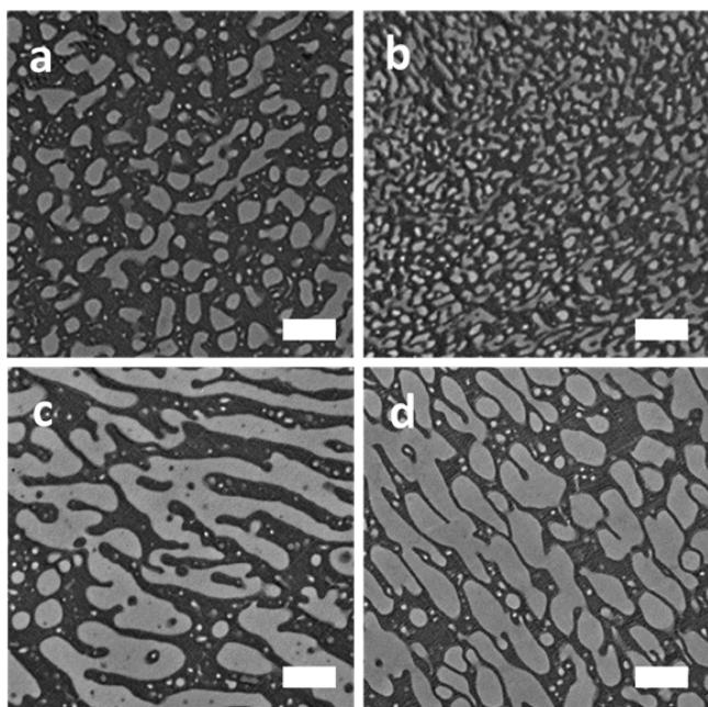
**Figure 5.** TEM micrographs demonstrating change in domain shape of PS/PMMA blends with 20 vol % SBM JPs in response to changes in blend composition: (a) 47:53, (b) 44:56, (c) 40:60, (d) 33:67 PS:PMMA. Scale bars represent 1 μm.
