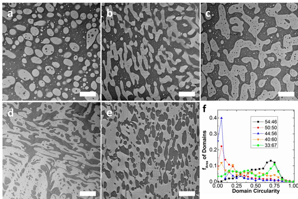
**Figure 4.** TEM micrographs demonstrating the change in domain shape of PS/PMMA blends with 8 vol % SBM JPs in response to changes in blend composition: (a) 54:46, (b) 50:50, (c) 44:56, (d) 40:60, and (e) 33:67 PS:PMMA. Scale bars represent 2 μm. (f) Histogram plot of the area-weighted fraction of dispersed domains as a function of their circularity, as determined by image analysis.
