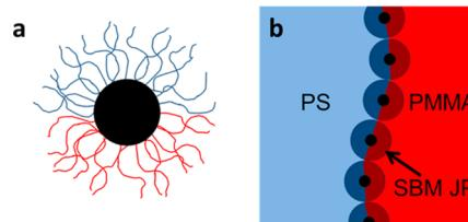
**Figure 1.** (a) Schematic representation of the structure of the SBM JPs, with cross-linked PB cores (black) and PS (blue) and PMMA (red) grafted chains. (b) Schematic representation of the assembly of the SBM JPs at the PS/PMMA interface.
